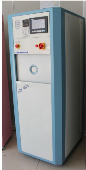
Figure 1. Existing Hydrogen Peroxide Plasma Sterilization Device of Teknomar Ltd. Co.
