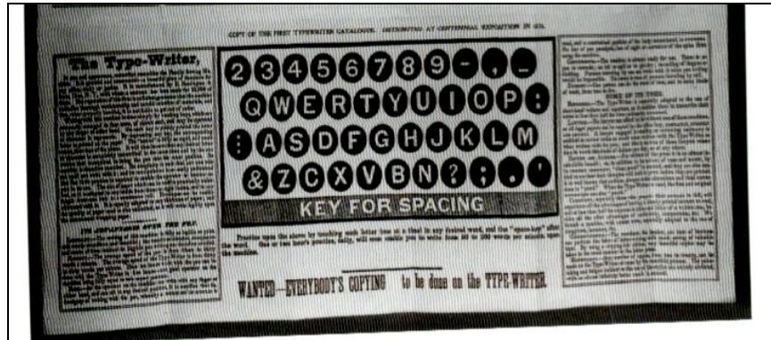
Figure 1: The QWERTY keyboard layout developed by Christopher Sholes. Russo, Thomas A. (2000). Office Collectibles: 100 Years of Business Technology . Atglen: Schiffer Publishing, 147.
