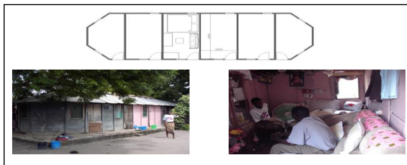
Figure 1. House Type 1. Walls and partitions are of “metal sheets”. A Room in this house type accommodates multiple functions and is occupied by one Household.
