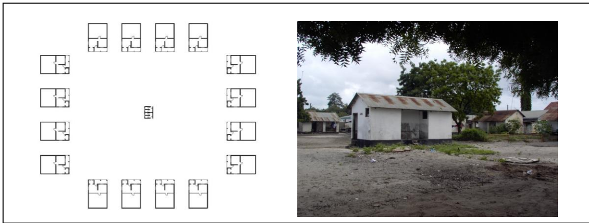
Figure3. The toilet building is centrally located being surrounded by sixteen type 2 houses.
